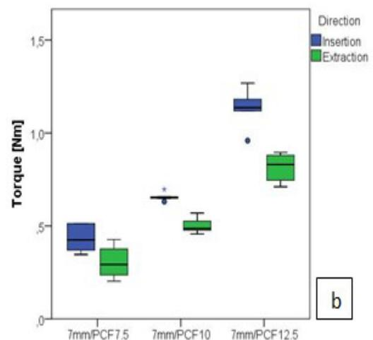
**Fig. 4a and 4b.** IT and ET by foam density and screw diameter. IT and ET for 6 mm (a) and 7 mm (b) diameter Neo pedicle screws in rigid polyurethane foam blocks of defined densities: 7.5 PCF (0.12 g/cc), 10 PCF (0.16 g/cc) and 12.5 PCF (0.19 g/cc); paired t-test: statistical significance for all pairs
