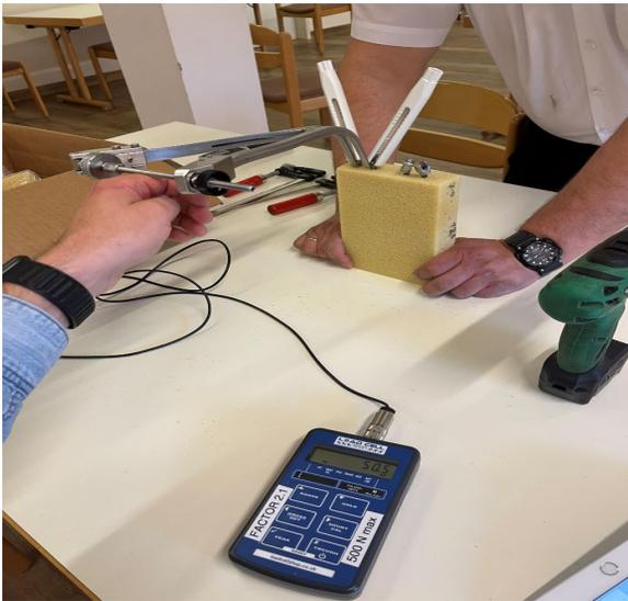
**Fig. 3.** Distraction across pedicle screws. Device which applies forces of 100N via Neo pedicle screws in polyurethane rigid foam blocks of defined density.
