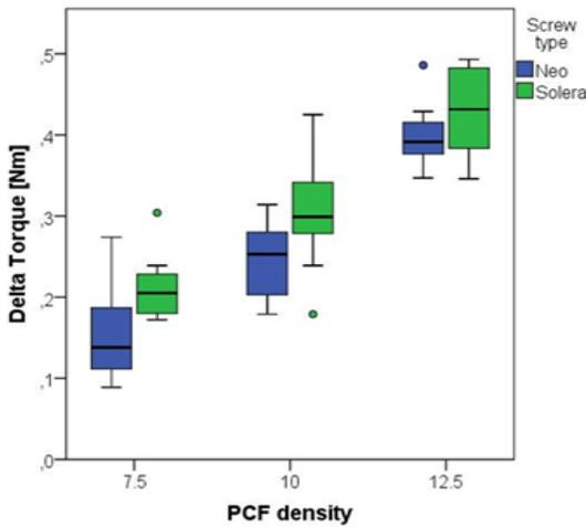
**Fig. 5.** Torque losses between IT and ET with distraction. Delta torque (IT vs. ET) for 6 mm Neo pedicle screws and 6.5 mm Solera pedicle screws in rigid polyurethane foam blocks of certain densities: (7.5 PCF (0.12 g/cc), 10 PCF (0.16 g/cc), and 12.5 PCF (0.19 g/cc)) when distraction forces of 100 N are applied to the pedicle screws
